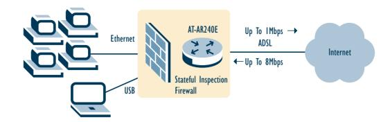
In the diagram above, the Ethernet and USB users share a single high-speed ADSL link to the Internet. They are also protected by a powerful Stateful Inspection Firewall which protects all LAN users from malicious attack, including Denial of Service (DoS) attacks. The AT-AR240E supports both Ethernet and USB ports; both can be operated simultaneously in routing mode.
